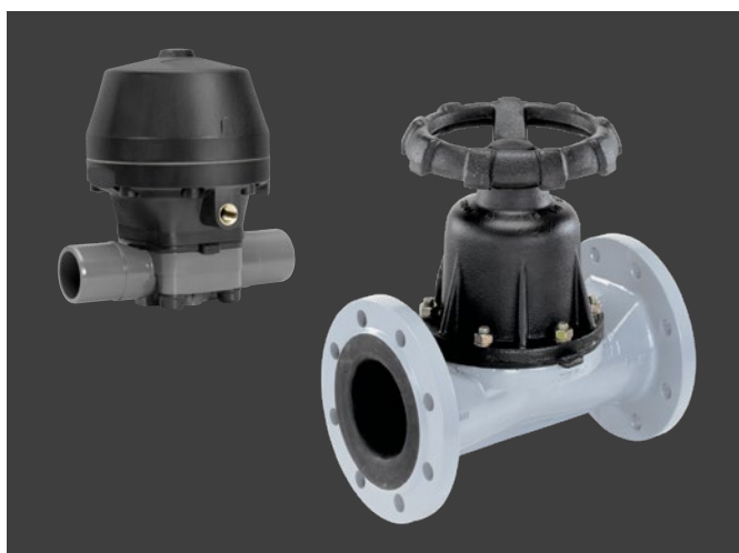
Fig. 4: Diaphragm valves in plastic or as full-bore variant are suitable especially for aggressive or particle-containing media
