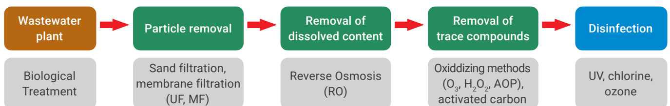
Fig.2: Schematic structure of the multi-barrier concept
